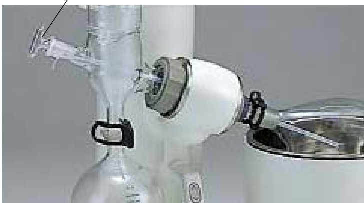
Sample induction cock (Teflon tube attached)
