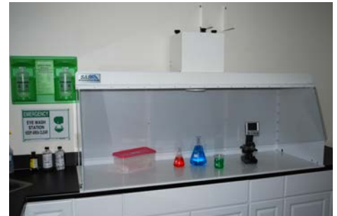
70" DCH provides chemical fume control.
