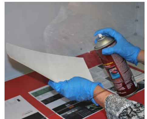
Close-up of operator safely spraying adhesive under a DSH.
