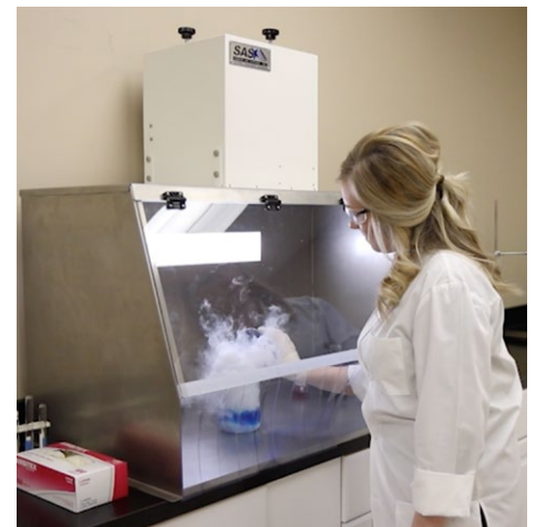
40" DCH provides fume control for various applications.
