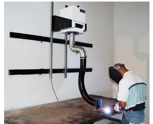
Model 300 Sky Sentry mounts on wall to free up needed benchtop space.
