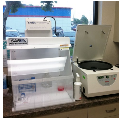
18" DCH provides fume control for a variety of laboratory applications.
