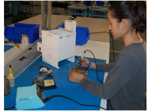
The operator is using the benchtop Model 200/225 Table Sentry to help protect herself from inhaling harmful soldering fumes.
