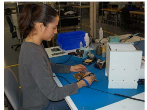
The operator is using the benchtop Model 200/225 Table Sentry to help protect herself from inhaling harmful soldering fumes.
