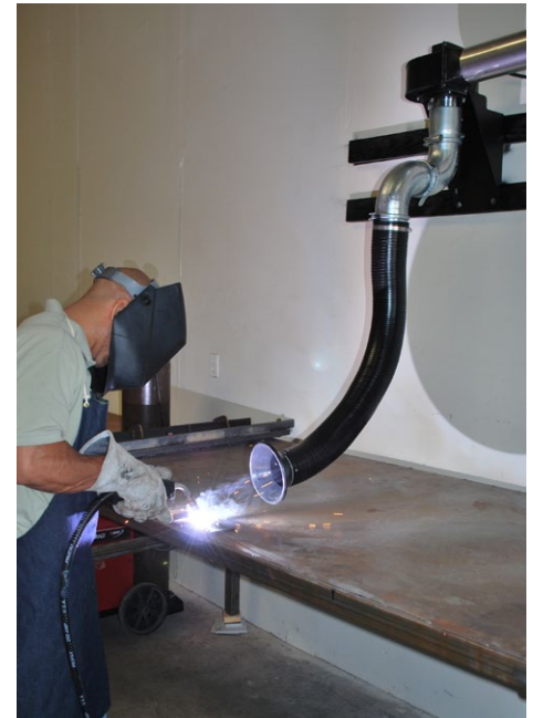
The Fan-Powered Flexible Fume Extraction Arm source captures fumes and can connect to existing ductwork.
