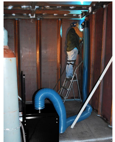
The extra flexible hose and magnetic capture hood helps welders extract fumes hand-free in hard-to-reach areas.
