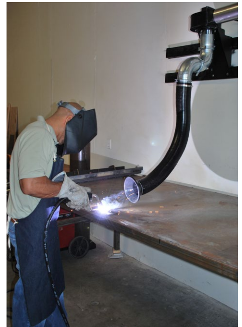
Non-Powered Flexible Fume Extraction Arm shown here extracting welding fumes using existing ductwork and fan (not included).
