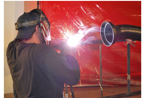
Black Flex Sentry Exhaust Hose is self-supportive and easy to maneuver allowing the operator to place the hood close to the fume and particulate source.
