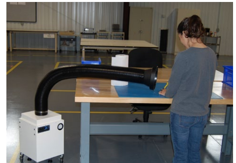
Black Flex Sentry Exhaust Hose is self-supportive and easy to maneuver allowing the operator to place the hood close to the fume and particulate source.
