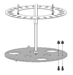
Rotate instrument stand so that the side with 2 nuts is on the right.
