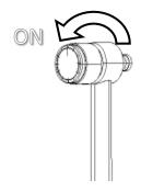
Turn the needle valve one revolution at each sample position being used.
