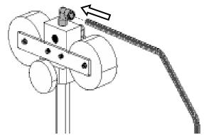
Connect the gas tube [J] into the swivel fitting [G] at the top of the instrument.
