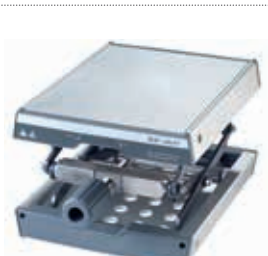
LABLIFT m Laboratory lifts lift and support small pieces of laboratory equipment and containers. A maximum weight of 7 kg (maximum dynamic load) can be lifted. Carrying weight: up to 25 kg (max load). The working height is between 70 mm and 300 mm Ident-No.: 0004022400
