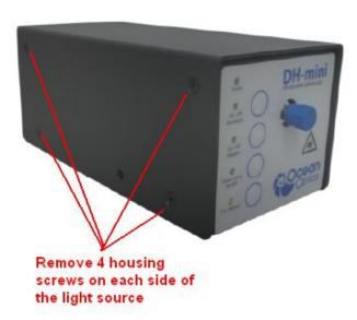
2. Lift the housing off of the light source.
