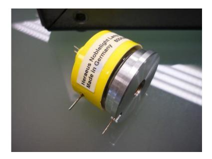
5. Insert a new bulb. Be careful to correctly align it with the connection holes on the PCB (3).
