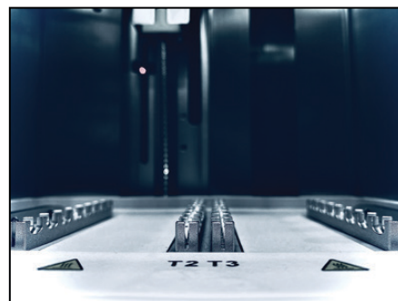
Heating block for lysis & elution
