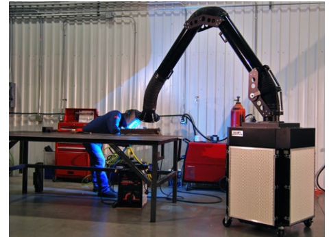
The 10' arm and capture hood allows the operator to capture most of the fumes and particulate close to the source.
