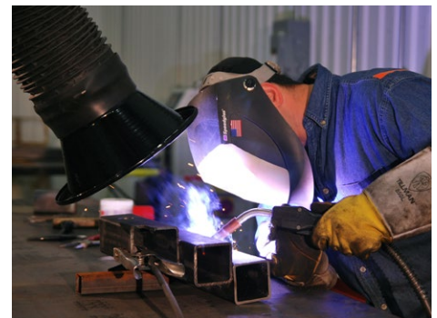
The 10' arm and capture hood allows the operator to capture most of the fumes and particulate close to the source.
