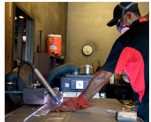
The operator placed the capture hose of the Python Industrial Fume Extractor close to his workstation to help capture particulate.
