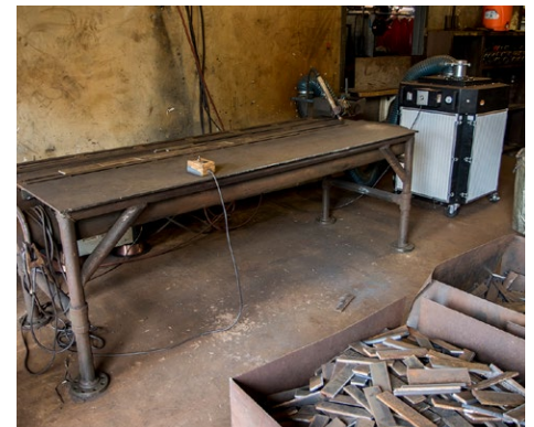
The operator placed the capture hose of the Python Industrial Fume Extractor close to his workstation to help capture particulate.
