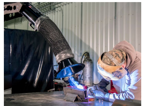
The 7' Heavy-Duty Arm can be easily maneuvered to source capture fumes.
