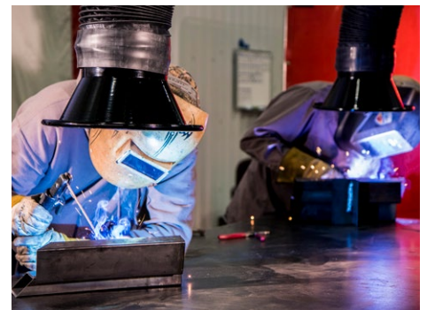
The 7' Heavy-Duty arms are easy to move for capturing fumes at the source.
