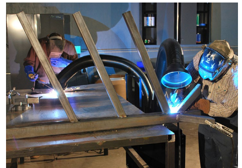
The Floor Sentry Double provides powerful fume extraction for two operators working near each other.
