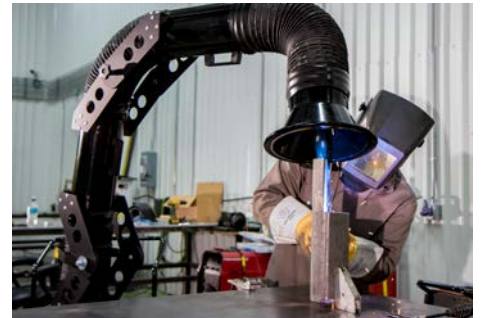
The Model 300 RuggedAir allows the operator to easily adjust the heavy-duty extractor arm to optimize extraction.
