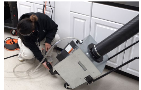
An employee conducting PAO testing on the Model 300 PAO Portable Fume Extractor by measuring the upstream and outlet concentration.
