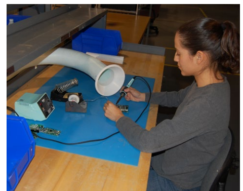
Two operators using the Floor Sentry Double unit to extract soldering fumes simultaneously.
