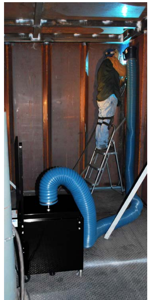
Model 200/225 Mini Fume Extractor is similar to the Model 400 Python Portable Floor Sentry which provides hands-free fume extraction for hard to reach areas and applications.
