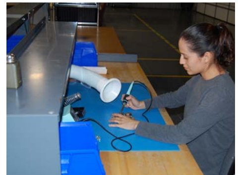
Model 200/225 Floor Sentry Double provides two operators with powerful fume extraction.
