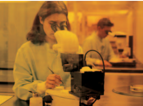
Leica S6 E with 38° viewing angle on transmitted-light stand
