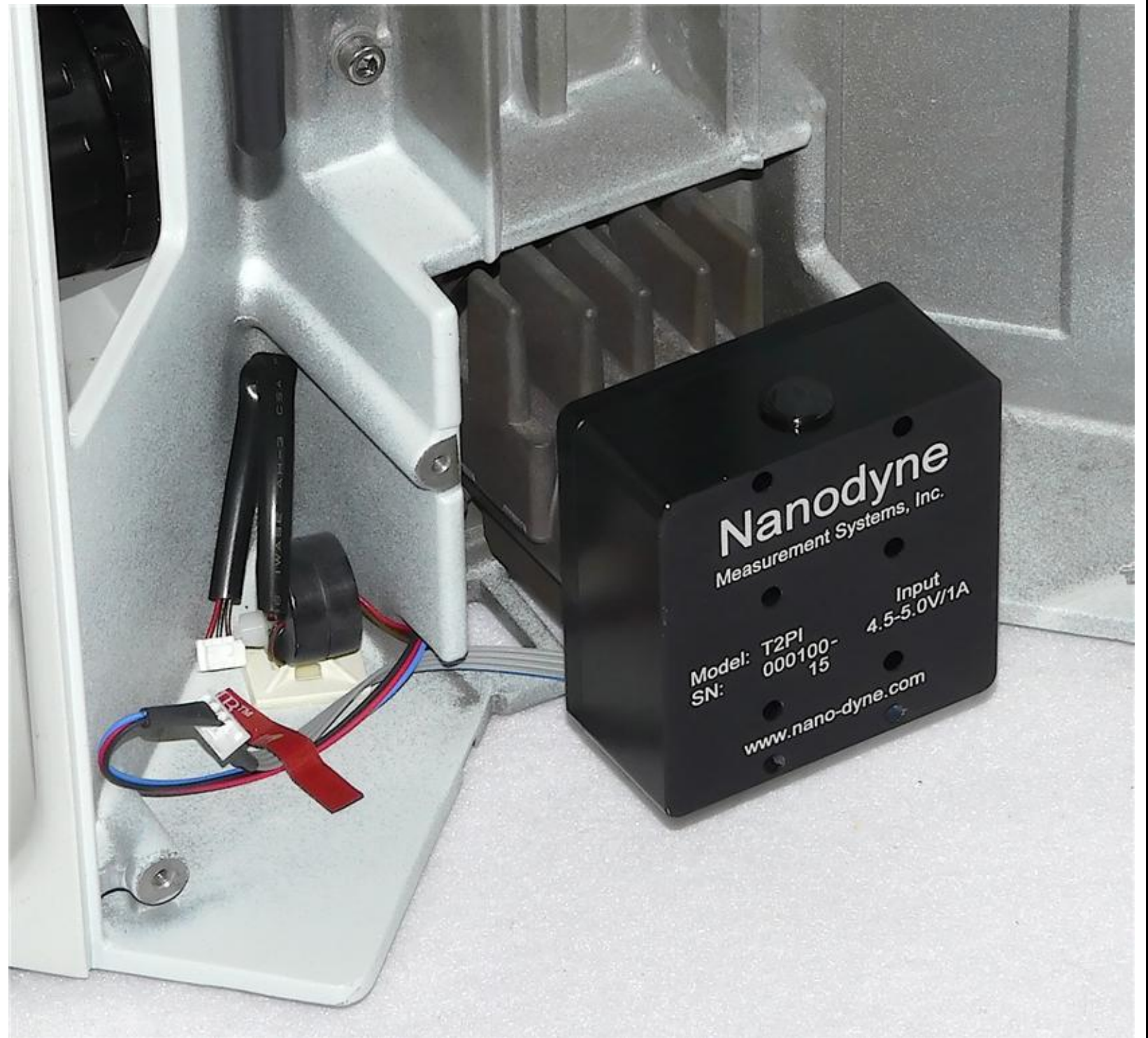
Step 7: Plug the Nanodyne illuminator into the microscope port, and secure the cables out of the way as shown above, using the strip of 3M VHB tape provided.
