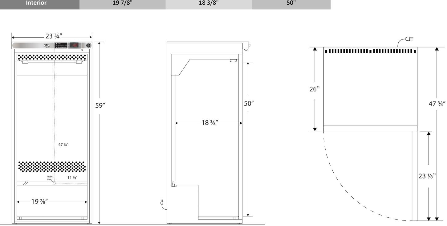
Note: This unit must have 4" clearance on sides and back for adequate ventilation
