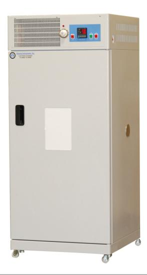
**The IncuMax IC500**, a 19.4 cu ft (550 liters) incubator from Amerex Instruments, features a PID microprocessor controller and a forced air circulation system to provide both exceptional temperature uniformity and rapid heat recovery throughout its stainless steel chamber. For stability, the casters are supplemented by leveling bolts. An electrical outlet enables low-wattage laboratory equipment to be operated inside the chamber.
