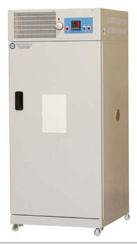
The IncuMax IC320R (320-liter, 11.3 cu ft) low-temperature incubator from Amerex features a microprocessor PID controllers and an efficient forced-air circulation system that provides both exceptional temperature uniformity and rapid heat recovery throughout its stainless steel chamber. It is suitable for applications from -5°C to 65°C. An electrical outlet enables small laboratory equipment to be operated inside the chamber and an independent over-temperature thermostat eliminates over-heating.
