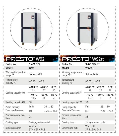
All data refers to the nominal voltage of 400 V, 3 Ph., 50 Hz and ambient temperature of  $+20\,^{\circ}$ C. Cooling capacity measured at max. pump stage. All pump data refers to a bath fluid with a specific density of 1 kg/dm³. Cooling capacity measured with Thermal HL ( $+200\,^{\circ}$ C) or Ethanol (except  $+200\,^{\circ}$ C)
