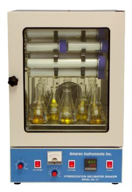
**Amerex's Model HS-111** is a versatile, compact hybridization oven that also functions as an incubator shaker. It incorporates a microprocessor temperature controller that together with a large and quiet circulating fan, assures uniform and precise temperature control. The large  $12.5^{\circ}$  x  $14.8^{\circ}$  double-pane glass window enables one to clearly and easily observe the inside of the entire stainless steel chamber.
