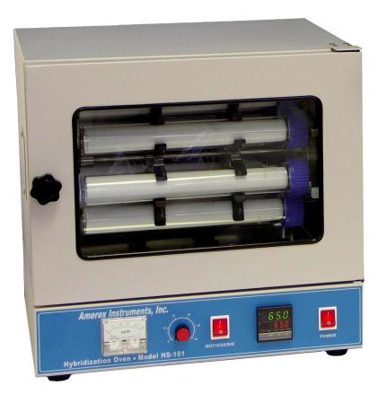
**Amerex's Model HS-101** is a compact, bench-top hybridization oven. It incorporates a microprocessor temperature controller that, together with a large and quiet circulating fan, assures uniform and precise temperature control. The large 12.5" x 14.8" double- paned glass window enables one to clearly and easily observe the inside of the entire stainless steel chamber. An analog panel meter displays the RPM of the rotisserie.
