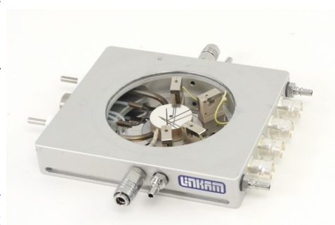
HFS600E-PB4 heating/freezing stage showing the 4 gold-tipped Tungsten probes.
