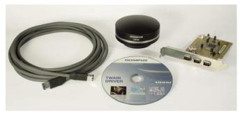
The DP25 digital camera system includes: camera head, PCI FireWire $^{\text{TM}}$  card, FireWire $^{\text{TM}}$  cable, and CD-ROM (TWAIN driver, a basic image acquisition software)
