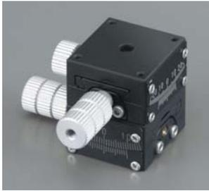
■ High cost performance gonio stage which dovetail system is adapted for a travel guide, and worm gear system is adapted for feeding mechanism. Ideal for use in R&D, integrating device and much more.
