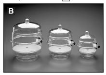
These rugged vacuum desiccators are molded of clear polycarbonate (NOTE: The white base on models F42010-0000,F42020-0000, F42025-0000 is polypropylene). The stopcock body is made of polypropylene, the plug and washer are made of TEFLON $^{\circ}$ , and the 0-ring is neoprene.
