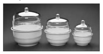
The Non-Vacuum Desiccator is used as a drying chamber for such items as thin layer chromatography plates, dried materials and chemical standards. The perforated plate rests on the inner ledge in the desiccator bottom. Samples are placed on top of the plate.
