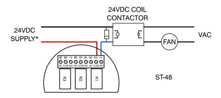
**NOTE**: ENSURE CONTACTOR CHOSEN HAS CORRECT COIL VOLTAGE AND IS CURRENT-RATED FOR YOUR LOAD
