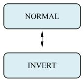
NOTE: When the CO<sub>2</sub> relay state is changed to INVERT, the internal horn will sound.
