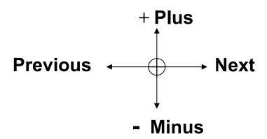
**Plus** – Pushing the joystick in this direction increases the value
