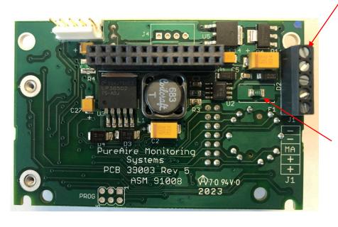
1. Power Analog output Terminal Block
