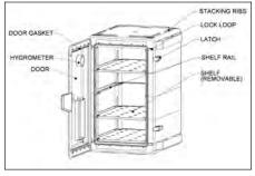
These cabinets have two door latches on the right side and hinges on the left. Leave space in front for the door to swing open. Place desiccant cartridges in the bottom of the cabinet and place the shelves into the cabinet starting at the bottom. Shelves
