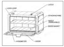
This cabinet is the same size as the 4.0 vertical but is wider and lower than the vertical cabinet. The door is hinged at the bottom and has two latches at the top. Two removable shelves are included. With the two shelves in place, the distance between the shelves is 110 mm
