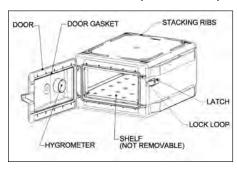
The cabinet should be placed on a horizontal surface with the door latch on the right. The space in front of the cabinet should be left clear to provide space for door opening.
