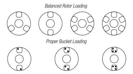
Buckets can be placed around the rotor in any of the rotor loading configurations shown.
